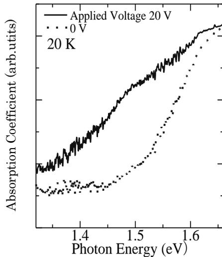
Fig. 1 Electrically induced change of absorption spectrum in Al-CuAlS<sub>2</sub> contact
